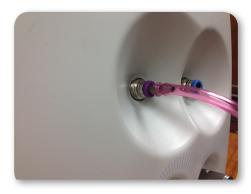
• Insert the other end of the tubing with the metal connector into the Diamond hand-piece, making sure it is secure.
