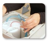
Press on the pink O-ring to remove the pink tube attached to the waste container from the machine.
