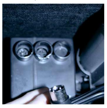
Check the connections to the T-connector make sure the cable is secure to the actuator
