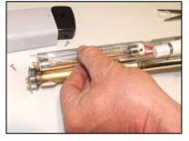
Optional: attach a new strap to secure the bulb. This is not absolutely necessary. The original strap was there to secure the bulb during shipping. Unless you are shipping your 3-in-1 to another location, this step is not required.
