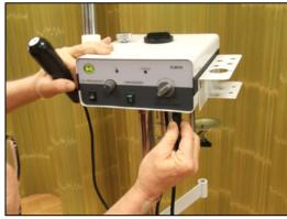
12. Plug the High Frequency Handle into its outlet.
