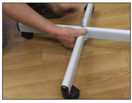
3. Insert the bolt (with washers in place) in the bottom of the Leg-Down portion of the Stand Base.
