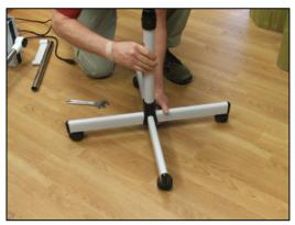
5. Slip the Pole Stand down over the Leg-Up portion of the Stand Base.
