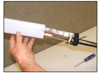
• To remove the bulb, cut the strap that was used to secure the bulb during shipping.
