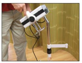
10. Place the Steamer Head on the Adjustment Tube.
