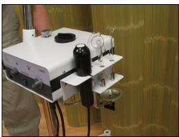
13. Insert the High Frequency Handle and probes into the holder.
