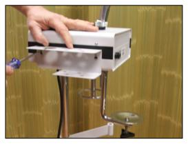
11. Loosen screws on the side of the steamer head slightly. Slip the holder for the high frequency handle and probes over the screws and tighten.
