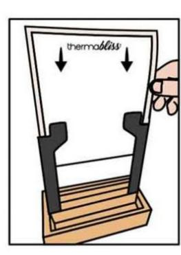
2. Insert Heater Pouch in center slot of chamber making sure it sits flat on the bottom.
