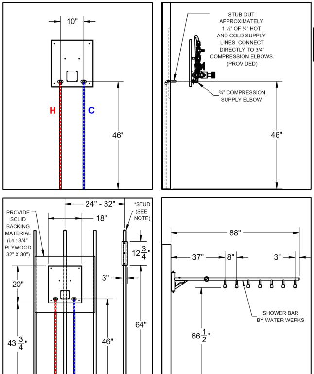
\* Adequate reinforcement backing is required. Use of metal stud is not sufficient reinforcement and is not recommended. Use of wooded stud is acceptable or equivalent. Failure to provide adequate reinforcement will result in damage to the Blast Vichy Shower and may cause bodily harm and serious injury.
