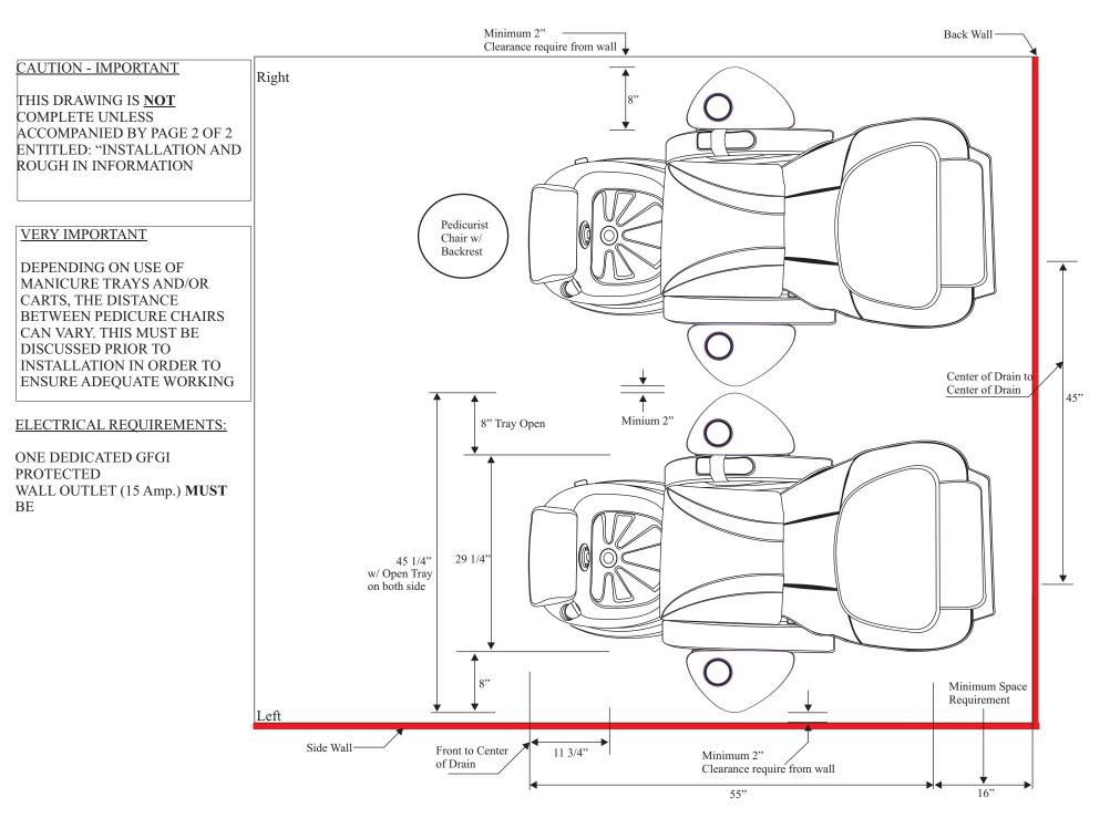
INSTALLATION DRAWING #2 Plumbing Rough - In (Back Wall Application) Page 2 of 2
