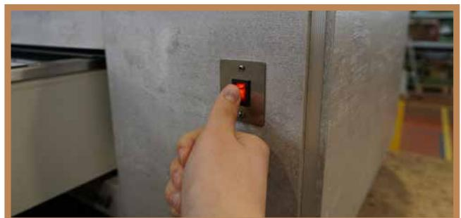
The drawer has two compartments: the bigger is heated, the smaller can be used for storage. To switch on/ switch off the drawer heating, press the ON / OFF button.
