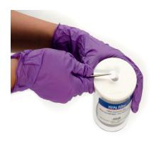
2. Remove the soiled disc and discard. Replace with a new filter disc.
