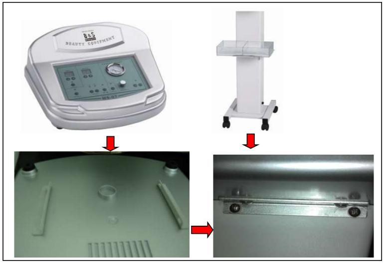
1. D-MS07 machine comes with two metal brackets pre-attached to the bottom of the unit. Carefully position the machine on top of the stand. Align the two screw holes in the brackets to the holes in the stand and tighten with a screwdriver.
