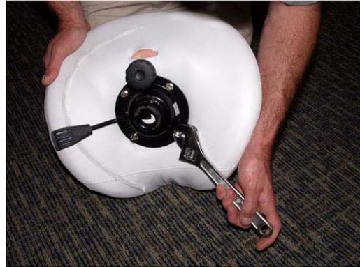
5. Lift the seat and place it on top of the pneumatic cylinder, inserting the cylinder into the opening in the stool seat. Press down firmly on the seat. Weight or applied pressure will serve to “pressure seal” these components.
