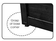
The *Premiere*™ weighs approximately 200 lbs. You will need 4 people working together if it is necessary to move the table. Never lift the table by grasping the table top as the table top is not designed to hold the weight of the base and you could damage the table and the electronics that run the tabletop.
