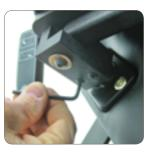
3. When you have achieved the desired height, tighten the two bottom set screws (turn clockwise).
