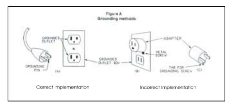
**DANGER-**Improper connection of the equipment-grounding conductor can result in a risk of electric shock. Check with a qualified electrician or service man if you are in doubt as to whether the product is properly grounded. Do not modify the plug provided with the product - if it will not fit the outlet, have a proper outlet installed by a qualified electrician.
