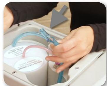
Press on the pink O-ring to remove the pink tube attached to the waste container from the machine.
