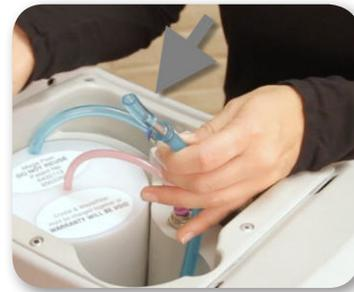
Attach the pink tube from the waste filter to the other end of the short blue tube from the spare parts kit which is already connected to the blue tube coming out of the machine.
