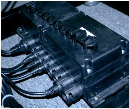
Check the connections to the T-connector make sure all cables are secure to actuator and plastic clamp is set.
