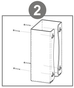
Dispenser should be mounted securely to a wall through keyholes in back with screws approved and provided by building maintenance.
