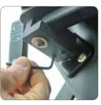
3. When you have achieved the desired height, tighten the two bottom set screws (turn clockwise).
