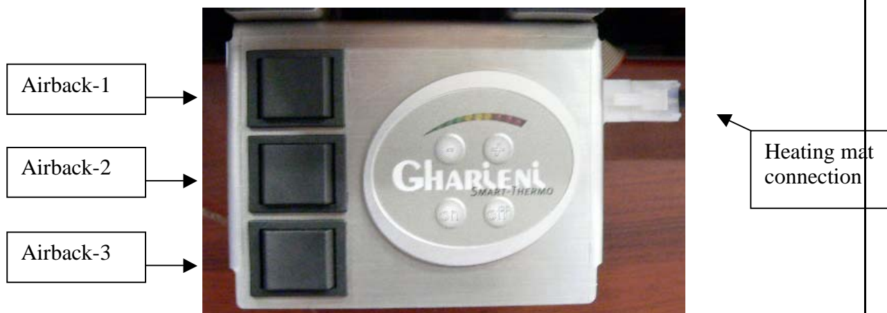
III. 6.5.1 Heating control panel
