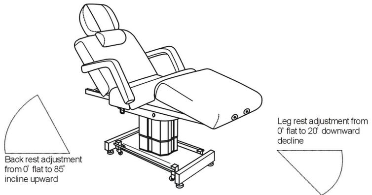
Back rest adjustment from 0° flat to 85° incline upward
