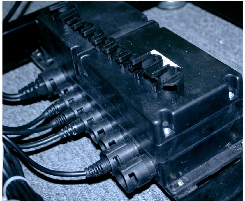
Check the connections to the T-connector make sure all cables are secure to actuator and plastic clamp is set.
