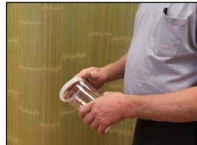
8. Slip the water jar up over the heating element and into place. Rotate the Metal Holding Plate under the Water jar. Then, turn the Plate Locking Knob to secure the plate under the Water Jar. Make sure the top of the Gasket creates a tight seal between the Water Jar and the Steamer. (*Note: the photos below show the arm for a magnifying lamp – not included with this steamer.*)
