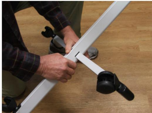
2. Insert the flat washer and lock washer on the 4" bolt and insert the assembled piece into the opening in the bottom of the stand.
