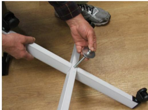
3. Turn the stand over and insert the Stand Connector into the top of the assembled unit. Note: you will need to hold the bolt assembly in place with your finger.
