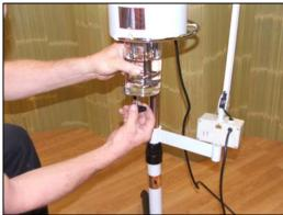
Note: You may put water in the jar prior to slipping the jar into place, or you may fill the jar through the fill port at the top of the steamer.
