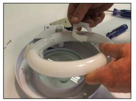
4. Disconnect the lamp at the receptacle. Replace the lamp.
