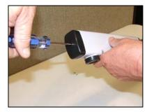
• Remove the screws found in side the top of the steamer arm.
