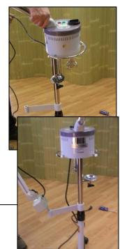
9. Insert the Magnifying Lamp into the end of the Magnifying Lamp Connector.
