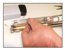
• Optional: attach a new strap to secure the bulb. This is not absolutely necessary. The original strap was there to secure the bulb during shipping. Unless you are shipping your 2-in-1 to another location, this step is not required.
