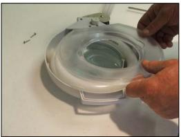
3. Lift the bulb up and remove the protective plastic braces.
