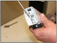
• Slide the housing off to expose the bulb and starter.
