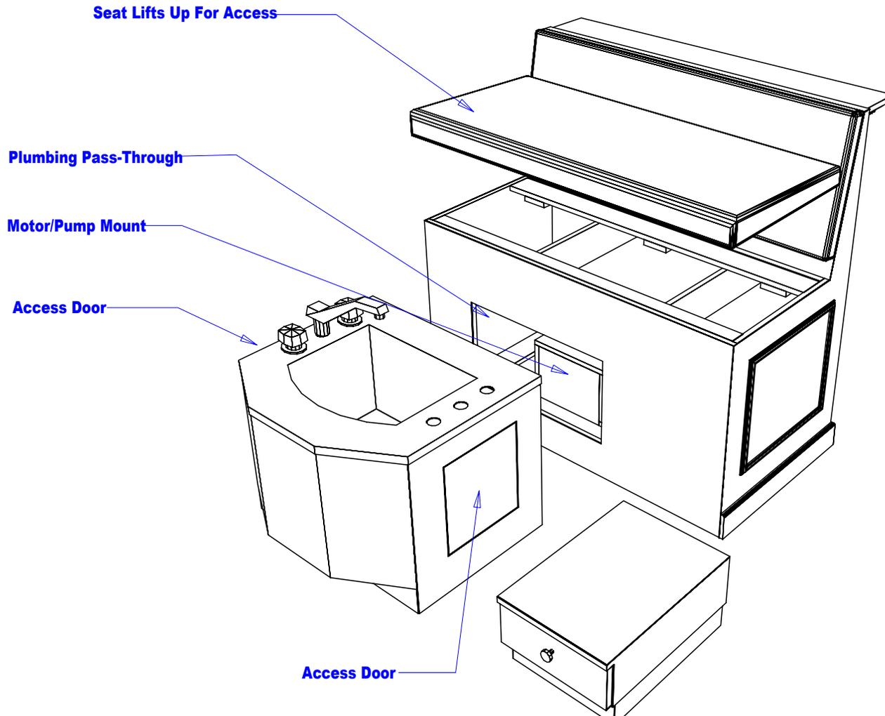
BOLT TOGETHER BENCH ASSY, SINK ASSY, AND STEP ASSY WITH PROVIDED FASTENERS.
