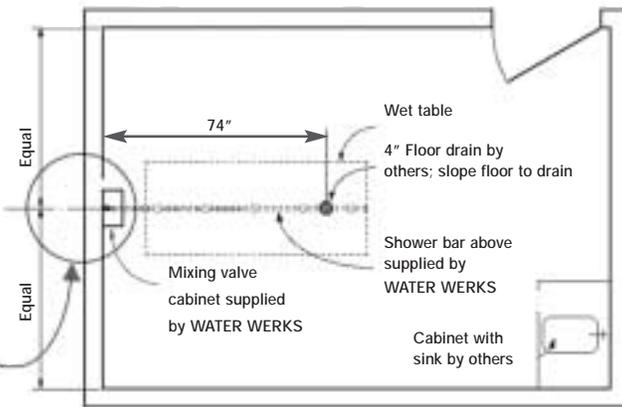
**Mixing Valve Cabinet Rough-In Elevation**
