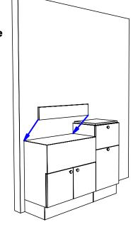
4. Adjacent cabinets and components should be assembled by fastening up through the bottom into the upper cabinet with the bolts provided. Tighten securely.
