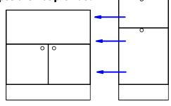
3. Attach loose backsplash to wall above assembled cabinets using contractor adhesive ("Liquid Nail").
