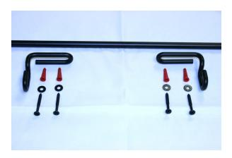
1) Drill 2 holes located 25" apart on surface where dispenser is to be mounted. Be sure that the holes are on a level, horizontal line. Drill 2 more holes 1/2" outside of the first 2 holes.
