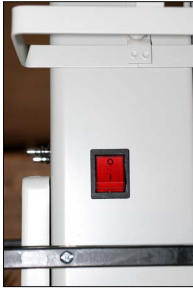
Main Power Switch (located on left hand side of the base)
