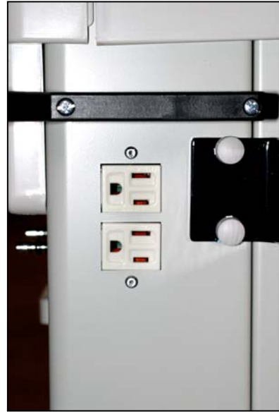
Outlets for Steamer and Mag Light (located on right hand side of the base)
